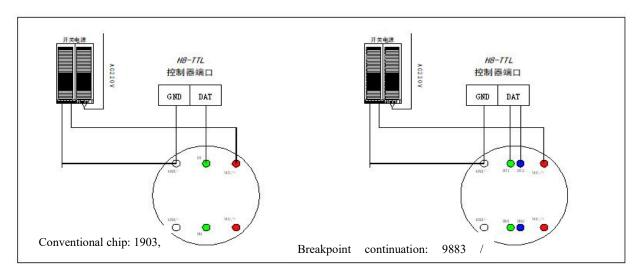
Requirements: 1, GND must be connected, to ensure that the ground line is the same.
