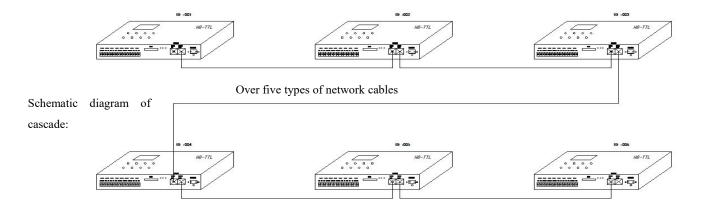
Note: A, cascade synchronization use crystal head network cable (568B parallel through).
