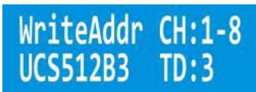
The representative is writing code, the writing code port is port 1 to 8, and the writing code chip is UCS512B3. TD represents channel, which is 3 channels.
