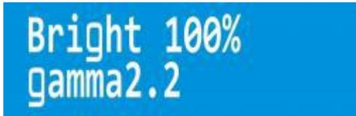
Step 3: Press  Press the speed +/-key (base 1) to switch the gamma value (1.0-5.0)  Press the mode +/-key (base 10) to adjust the corresponding value  Cycle / OK to save and return to the main screen.
