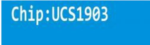
Step 3: Press
