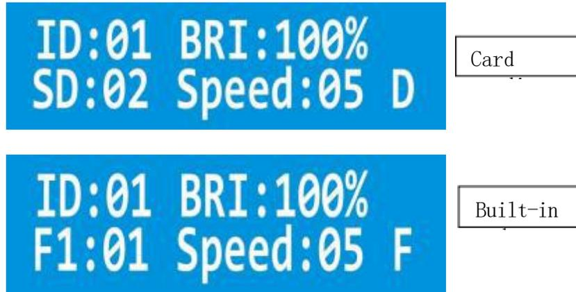
① ID: 01 represents the current controller number is 01, which is the first controller, and the maximum is 255.
