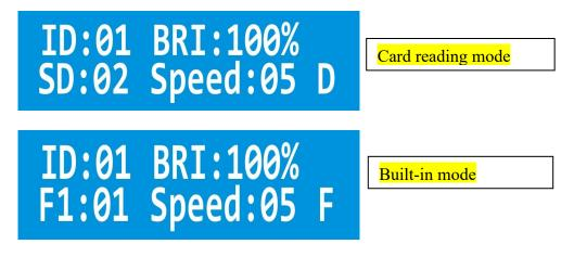
(1) ID: 01 represents that the number of the current controller is 01, which is the first controller, and the maximum is 255.
