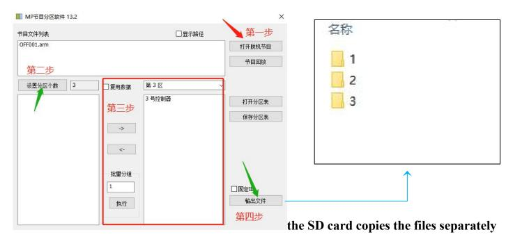
The controller SD card copies the corresponding files respectively:
